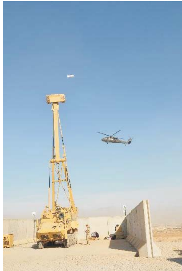
GAMB Radar mounted on a Piranha vehicle
