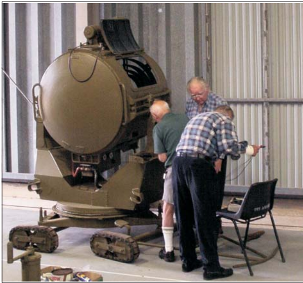
90 cm Searchlight. Original members of 67 AA Searchlight Battery who served during World War II, provide their expertise in the restoration of this 90 cm searchlight. It is now an operational light and used on special occasions.
