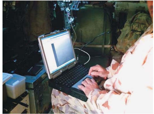
Figure 4. Tier II UAV Remove Viewing Terminal inside ASLAV
