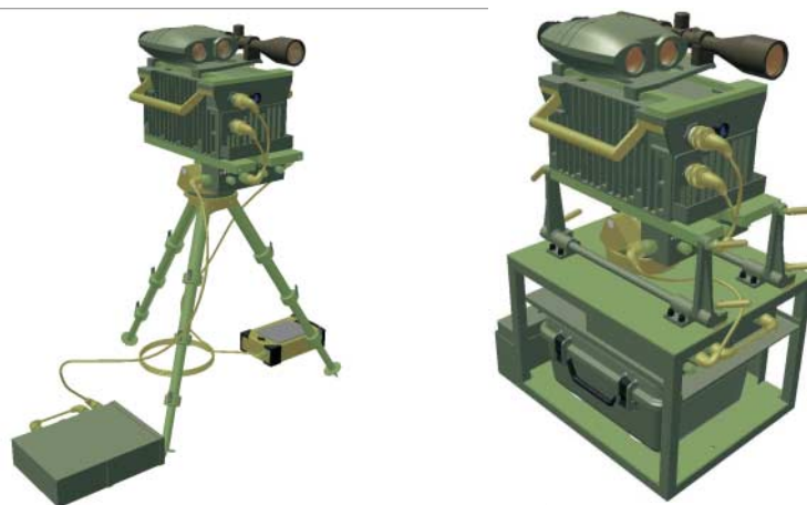
Schematics of the AOS in Remote (left) and Vehicle Mounted (right) Configurations
